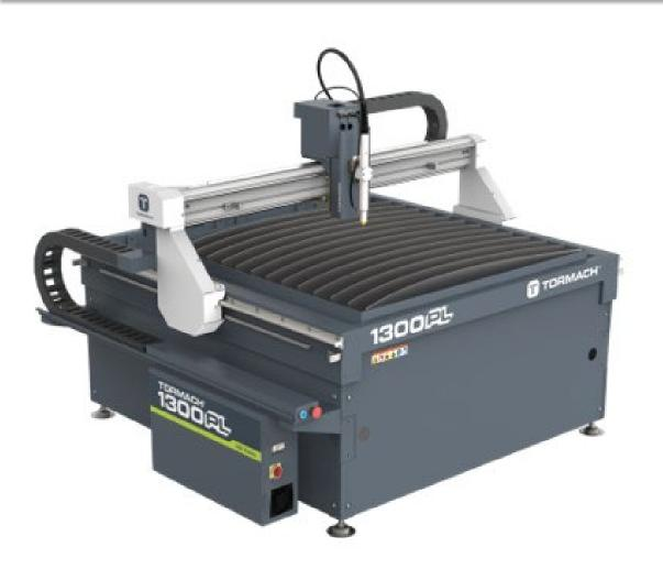
A Tormach 1300 PL CNC Plasma machine is easy to use, cuts any metal 2D sheet material into complex shapes to be made into 3D projects. This valuable training tool is one the Clover Park Advanced Manufacturing school is missing. Retail cost \$18,000
